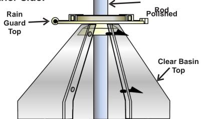
Drop joined Basin Top and Rain Guard Top into the slotted base.
